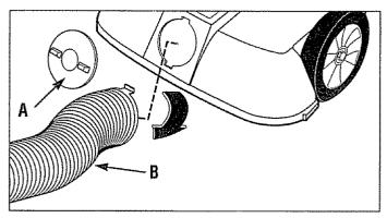
Figure 16: Remove vacuum inlet cap and install vacuum hose.
